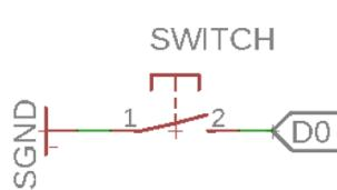
digital inputs D0-D8 are provided with a pull-up.
