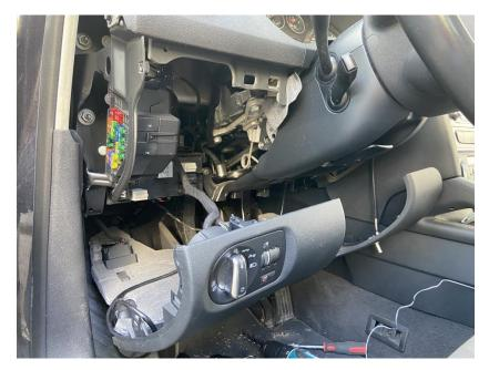
The place where you can position the rotary knob is only limited by the length of the cable. It would also go near the ashtray. We opted for the area under the dashboard.
