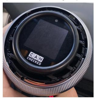
The glare ring is also remounted. Pay attention to the positioning of the locking lugs
