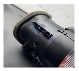
Now pass the display through the adapter ring. Then plug the 12 and six-pin Molex connectors into the display.
