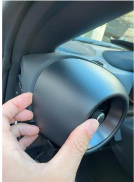
Once the screw has been removed, the entire air vent can be pulled towards the driver's seat and is prepared for installation in the next step.
