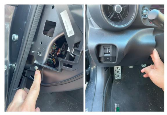
The entire fairing can then be pulled towards the driver's seat and thus released. ATTENTION: There are still 2 cables on the fairing, these can be disengaged and disconnected by finger.
