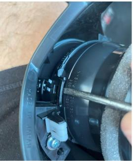
After successful removal of the air vent, your air vent will look something like the picture below. If this is the case, you can slide your display with our holder into your disassembled air vent and snap it back into place. You will find a picture of the panel locked into the air vent in the next chapter.
