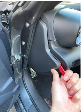
Phillips screw is revealed under the side cover. This must be removed.
