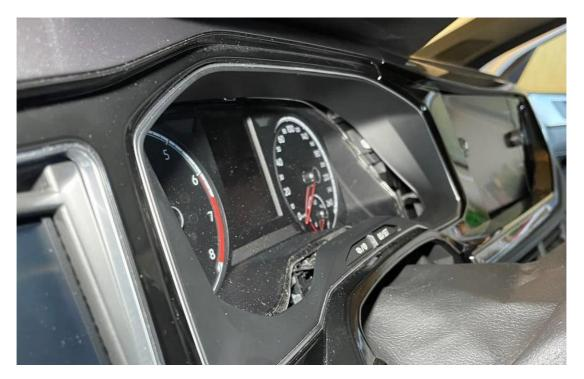
The next step is to complete the steering column cover. This is locked in place under the speedometer (red) and then pushed down towards the steering wheel (blue).
