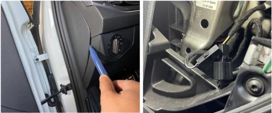
The next step is to remove the cover of the steering column. This is also only clipped and can be released by deliberate levering.
