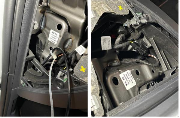
Now all that remains is to clip the side trim back in place and secure the excess length of OBD cable with cable ties at the top of the footwell. DONE!
