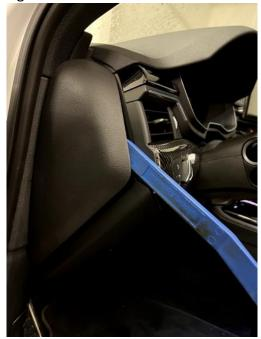
In the second step, the three M6 screws (one from the side and two from the bottom) must be removed.
