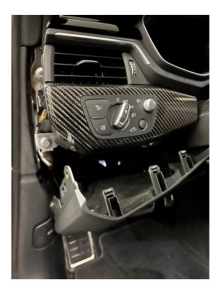
The aperture is held from below with a Torx screw. This must also be removed in order to be able to carefully lever off the aperture afterwards.
