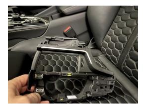
Now insert the display from behind in the same position and use the latching noses. First position the upper part, then the lower part and then snap all three Clips into place.
