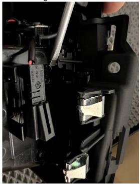
On the underside there is also a latching nose. If this is also loosened, the ventilation grille can be removed from the shaft.
