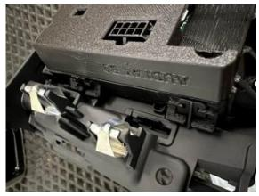
Important during installation is a clean finish of the top of the display. For an optimal fit, the front cutout must be enlarged a little with a cutter knife until the display fits perfectly.
