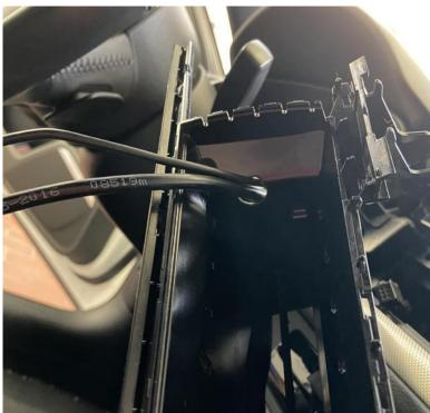
Pin the pins into the two connectors (A=8x, B=10x). Please pay attention to the enclosed note from the connection cable and the quickstart guide of the display.
