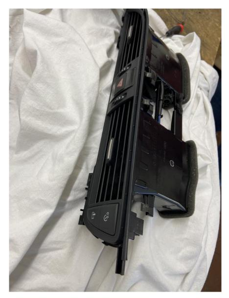
Now we dismantle the black-matte plastic panel. For this purpose, the retaining noses must be unlocked:
