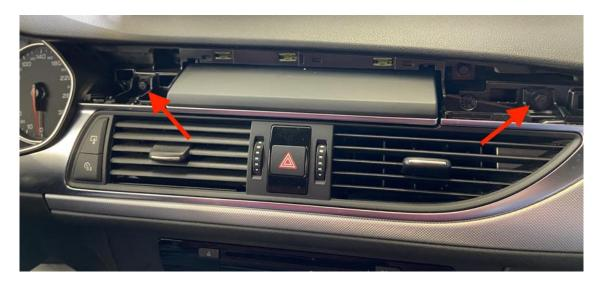
Lever the fairing under the speedometer a little upwards so that you can remove the ventilation unit:
