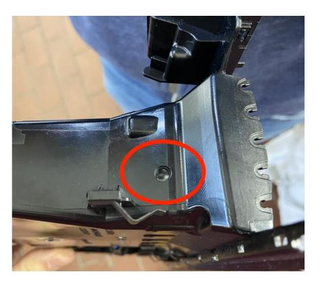
We thread the OBD cable from the OBD socket at the bottom left of the driver's footwell with the pulling aid for ventilation. We first led the pulling aid from the ventilation downwards, fastened the cable and then slowly pulled it upwards.
