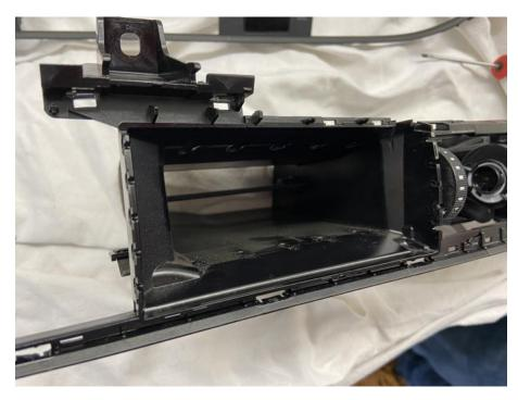
Laterally, we drill one large or two small holes: for the OBD connection cable and for the USB cable:
