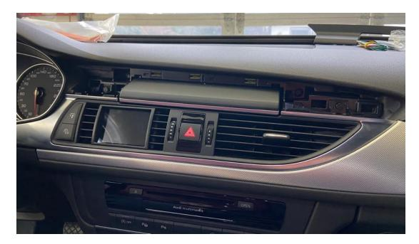
At the end, insert the top cover and press with the flat hand until it clicks into place.
