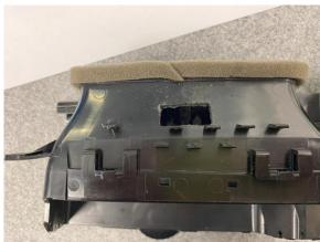
Now you can run the USB and CANchecked cable through the hole, connect it to the display and clip the vent insert into position.
