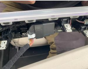
Now the junction box must be exposed. To do this, remove the cover of the passenger footwell. To do this, turn the two holders by 90° and then fold the cover down. Disconnect the footwell lighting and remove the cover.
