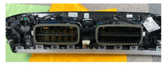
Once you have removed the two ventilation ducts, you can now separate them from each other and remove the louvers from the part on the driver's side in order to drill 2 holes in the ventilation duct with the 10mm drill bit. The holes should be close together, so you can work them out to a slotted hole afterwards with the small file. This should look like this:
