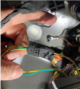
This completes the connection of Can High and Can Low. The next step is the connection of the ground and 12V ignition plus. The ground is connected to one of the ground points via a ring terminal. To loosen this, a 10mm nut is needed. After the ring cable lug is connected to the ground point, please tighten the nut again!
