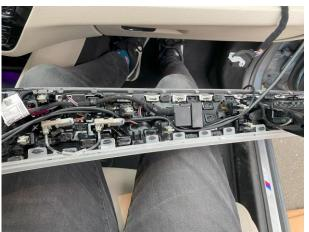
Now the bezel can be clipped into position once you have reconnected the two connectors. The rest of the assembly is done in reverse order.
