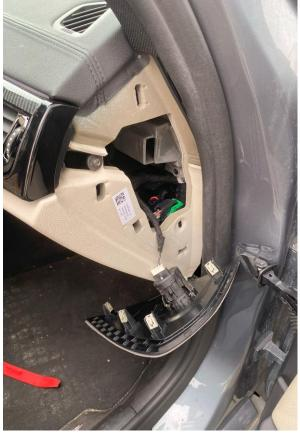
Now the Torx screw that appears must be unscrewed and the entire strip, including the ventilation nozzle, can be levered off, starting at the side and going around.
