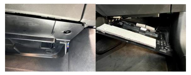
Carefully pull up the sill cover and remove it in the same way. If the clips get stuck in the body, remove them with pliers and clip them back into the trim.
