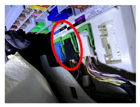
To release the connector, push in the latching lug and flip the lever. When the lever is turned, the connector is lifted out of the board. Now you can use a fine screwdriver to release the latch on both sides of the pin carriers and push the pin carriers out of the housing.
