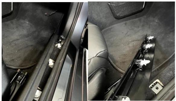
Now carefully unclip the side cover on the right side of the passenger footwell and set it aside, exposing the junction box underneath the carpet.
