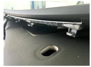
The unhooked Curved Display can now be placed on the dashboard.
