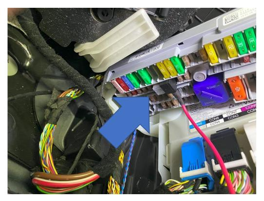
Now you just have to connect the connector housing of the black and red wire to the pigtail that you previously plugged into the ground point and the fuse holder.
