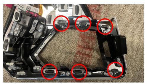
Once the caulking points are removed, you can push the plastic trim of the panel out towards the front.
