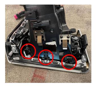
Now you need to use a Dremel to open up the bezel at the following caulking points so that you can then mount the insert.
