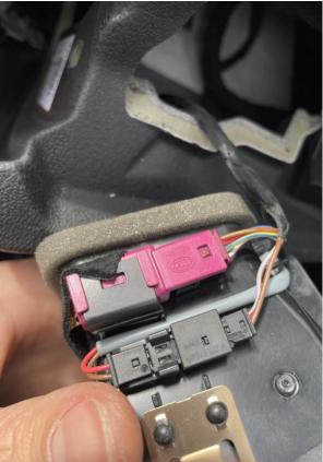
Now you need to unlock the two connectors on the bottom of the nozzle to remove the nozzle.
