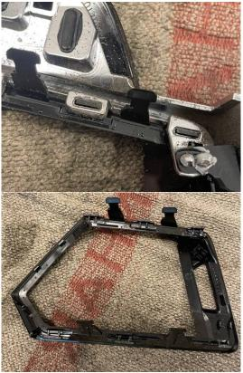
If you were able to remove the original insert from your panel, you can now insert the CANchecked insert starting from the former adjustment wheel and then clip it in towards the high-gloss trim.
