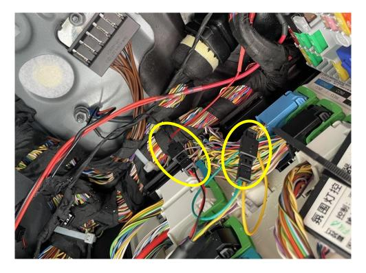
Now you only have to connect the USB and the CANchecked harness to your display, clip in the bezel and check the display for function. If this is given you can complete the vehicle and you are done.
