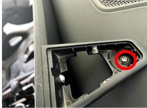
Once these steps have been taken, the Curved Display can be pushed upwards out of the hooking as a complete unit. (To do this, first pull the entire display backwards and
