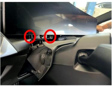
The next step is the rear support on the passenger side. The trim must be levered off and then the two TX20 screws loosened (Attention: screws have different lengths!) Then the support can be removed.
