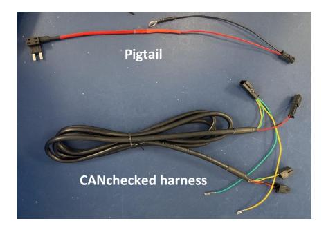
After you have laid the cable harness in the direction of the junction box, you must now pin the two loose wires. Can High (green) and Can Low (yellow) must both be pinned into connector 8.
