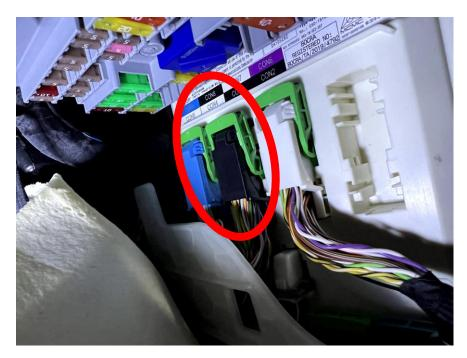
To release the **connector 8**, push in the latching lug and flip the lever. When the lever is turned, the connector is lifted out of the board. Now you can use a fine screwdriver to release the latch on both sides of the pin carriers and push the pin carriers out of the housing.
