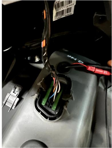
Since OBD and the USB cable, you now lay from the OBD socket towards the air vent in the center console. Store the USB cable so that you can easily plug it later for settings and updates.
