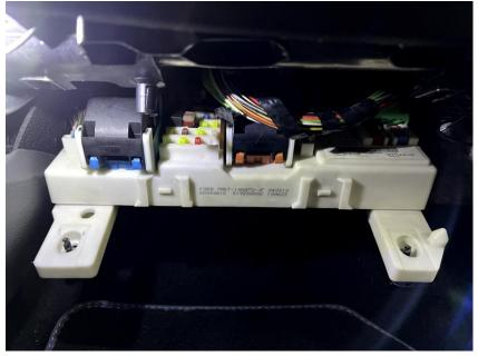
The supplied fuse adapter is now plugged into the exposed fuse holder and the additional cable is crimped. The remote fuse is plugged into the adapter.
