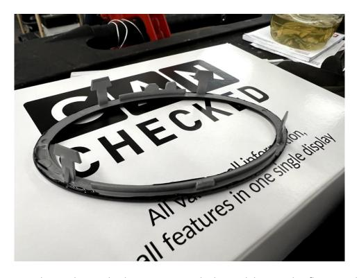
In the second step, the two latching noses must be levered down with a flat screwdriver in order to be able to pull out the channel.
