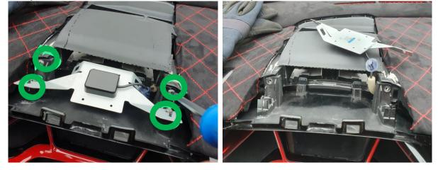
Now dismantle the fairing under the steering wheel by pulling it towards you. Don't forget to unplug the plugs on the left side and the plug and hose on the right. Then you canpull the hood side panel away to the left.
