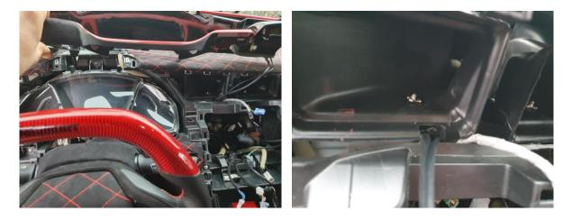
The red cable of the OBD connector must be wired to the fuse adapter in a slot with ignition plus.
