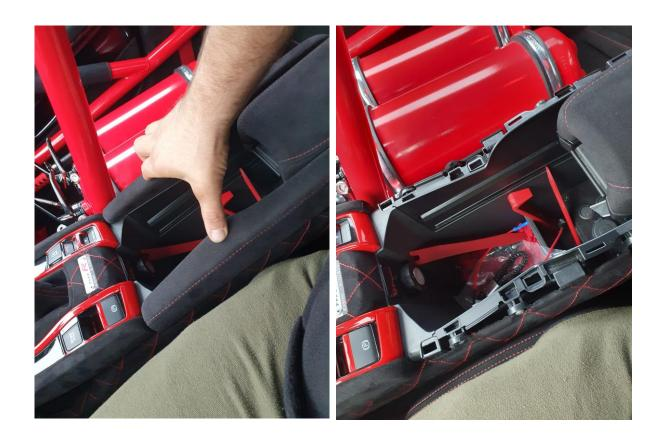
In the second step, the side panel around the gear knob must be dismantled. To do this, please pull it upwards.
