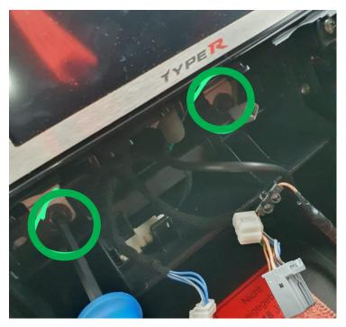
After the screws are loosened, the screen can be grabbed left and right and pulled out of the shaft vigorously. Again, please remove all rear plugs. Then the fairing can be carefully pulled towards you.
