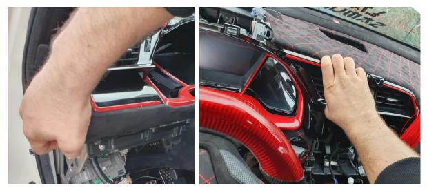
Pull out the cover so that you can release the rear plug for the hazard warning light switch. If you have solved this, you can remove the aperture completely.
