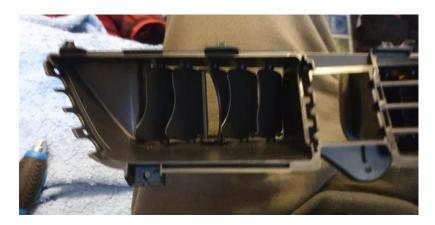
Now you can run the cables from behind through the slats and plug them into your data display. And push it into position.
