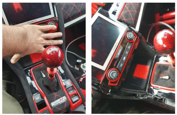
Now the ventilation unit can be grabbed on both sides and pulled towards you. The plugs on the back can then be carefully removed and the ventilation unit set aside.
