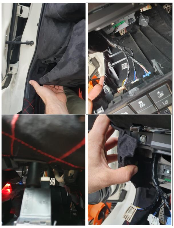
Once you are ready, you can now carefully pull the speedometer cover with the ventilation unit piece by piece towards you.
