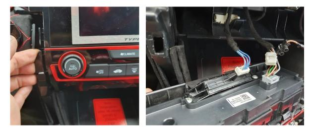
Now the two screws holding the screen can be loosened:
