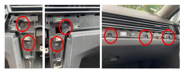
The ventilation nozzle can then be pulled out of the dashboard across its entire width and then the 3 connectors of the wiring harness can be disconnected to remove the nozzle completely.
