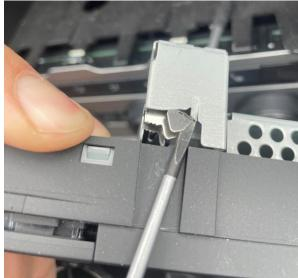
If the radio is also removed, the 7 TX20 screws holding the air vents must be removed:
