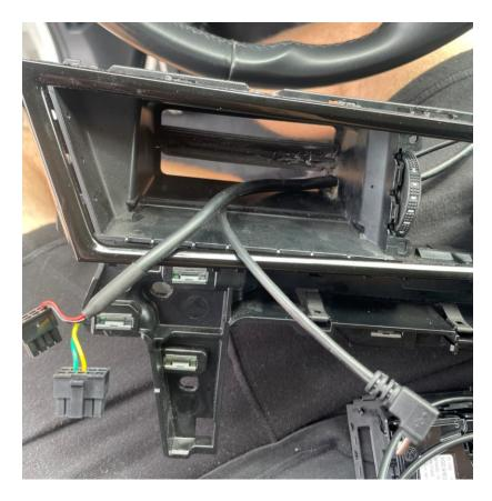
The cables can then be connected, and the trim can be inserted into the ventilation shaft. Then the clock and the decorative frame are clipped back into position.
