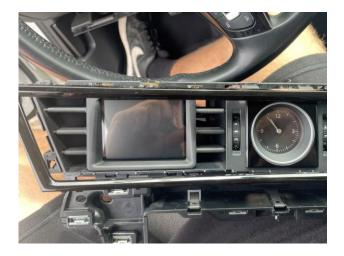
When you are ready, you can push the entire ventilation unit back into the dashboard, making sure that the cables are correctly positioned. Please also reconnect the previously disconnected plugs! Then push the radio back into the shaft.
