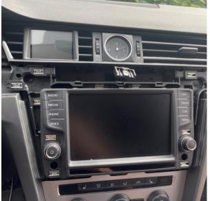
Now clip the trim around the radio and the speedometer back in place, plug in the hazard light switch and clip the remaining trim into position.
