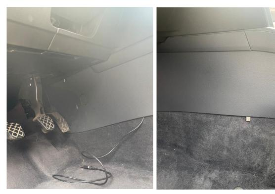
The OBD cable is stowed above the footwell trim, fed out of the clearance for the OBD connector and then plugged in there:
