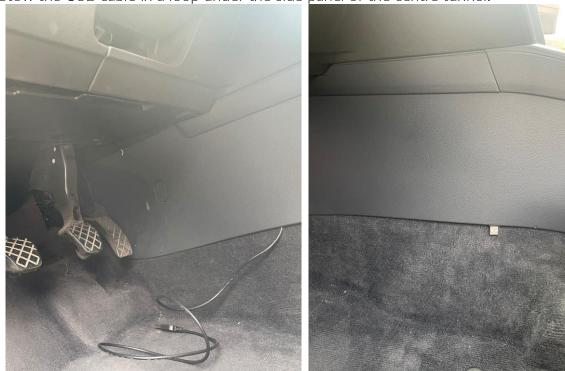
The OBD cable is stowed above the footwell trim, fed out of the clearance for the OBD connector and then plugged in there:
