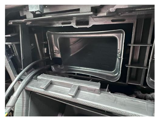
Now all that is left to do is to run the USB cable and the OBD cable from the driver's footwell up towards the air vent. Some stiff wire can make the work much easier. Once at the top, the cables can be routed through the panel and connected to the display.
