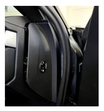
Now we lead a wire through from the side to the position of the speaker. Here you can shine through, have an orientation and see if the wire takes the right direction.
