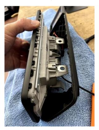
This is where the CANchecked panel comes in. The new bezel is not designed to be clipped in and out multiple times. After loosening and fastening, the proper fit can no longer be guaranteed. Once everything is in place, the bezel can be carefully clipped in place with your hands. Be careful not to pinch the cables from the display.
