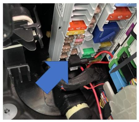
Now you just have to connect the connector housing of the black and red wire to the pigtail that you previously plugged into the ground point and the fuse holder.
