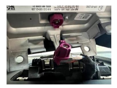
Remove the rear bezel of the screen with a plastic wedge. Start at the bottom and work your way to the sides.
