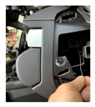
At the end of the wire, we fix the cables and carefully pull them through. On the screen side, the CANchecked wire harness is passed through together with the screen's central connector.
