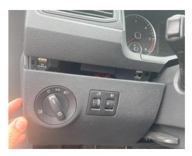
Once you have loosened the fairing, you have a clear view of the red plug of the gateway. This is where the enclosed adapter wiring harness is plugged in. To loosen the plug, please press down the tab and then unplug the plug and insert the wiring harness in between.
