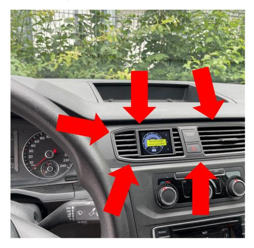
Once the ventilation unit is out, you can route the two plugs of the adapter wiring harness below the steering column towards the center console to the hole in the dashboard. Move the USB from top to bottom so that it ends next to the side footwell trim (you can hide it here later. Once this is done, it should look like this:
