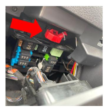
Now look at the next picture: Now use the mounting tool to carefully pry out the fairing that holds the middle air vents at the places marked with an arrow all around.
