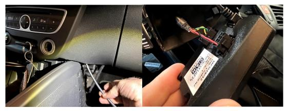
Now also plug the USB cable into the display, run it through the slotted hole and lay it downwards, where it can be hidden under the side panel of the center tunnel, for example.
