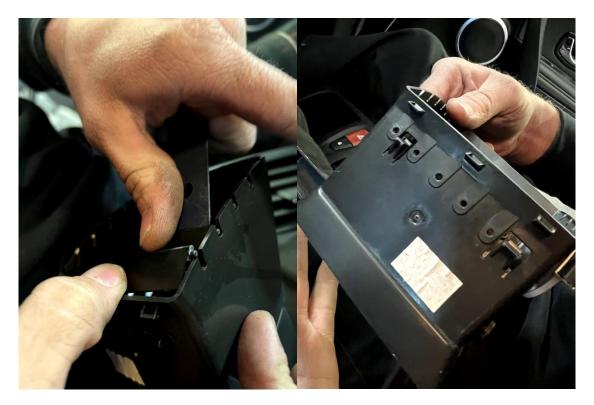
I use the 10mm drill to drill 2 holes in the ventilation duct. The holes should be close together so that you can work them out into a slotted hole afterwards with the small file . This should look something like this:
