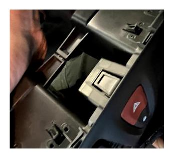
Now all you have to do is push the panel and display back into the dashboard, insert the OBD plug into the socket and hide the rest of the cable behind the panel, and you're done.
