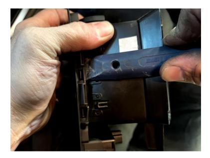
The two channels are still connected in the middle – this connection must also be loosened.
