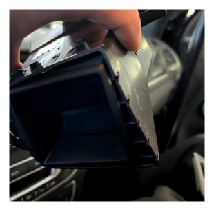
Then clip the ventilation duct back into its original position and reconnect the two ducts left/right.
