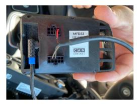
Please **URGENTLY** check the assignment of the cable. The OBD cable comes with a note with the assignment.
