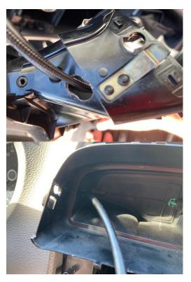
Next, slide the pins into the plugs of the display. Here you have to pay attention to the correct position and that the pin clicks easily. Then plug the plugs into the display. Increased caution is required with the USB cable. The USB socket is very small and the cable must be inserted very carefully. Damage to the USB socket must be avoided at all costs and is not covered by the warranty.
