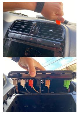
Clip off the screen on the upper tabs and remove the buttons as well. Please be careful with the metallic retaining brackets (red arrows) on the buttons. They like to slip off and disappear into the depth of the center console.
