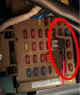
We've opted for the second slot from the right in the middle row in this guide. If there is already a fuse here, it must be removed and plugged into the adapter. Then plug the adapter to the fuse box.
