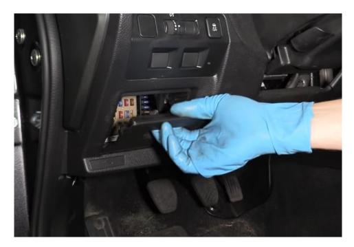
Now use the mounting tool to carefully pry out the trim that holds the air vents.
