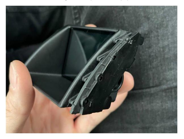
Once you've made it this far, plug the previously laid OBD and USB cable through the hole in the ventilation duct, plug it into the display and can insert the cover with the display into the ventilation duct and clip it together.
