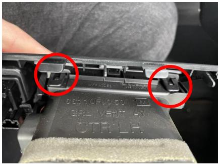
Once you have loosened the clips and pulled the ventilation duct backwards, the whole thing should look like from the next picture. The light-colored plastic frame remains in position and does not need to be dismantled.
