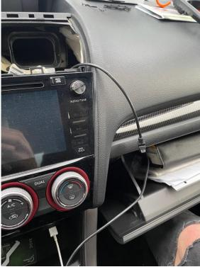
Plug the OBD plug into the OBD socket and route the separate red wire from bottom to top towards the fuse box, crimp it with the enclosed fuse adapter and plug it into a slot with 12V ignition plus.
