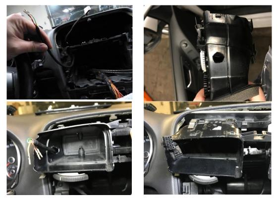
Next, slide the pins into the connectors of the display. Here it is important to ensure the correct position and that the pin clicks into place slightly. The assignment can be found in the note for the OBD cable:
