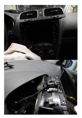
Unplug the white plug and loosen the cable fastening as well. Now the ventilation panel can be completely removed.
